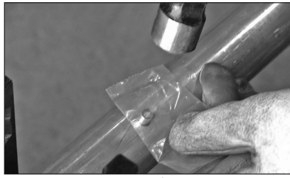
FIGURE 10b: Filler plug left in plastic bag is easier to insert with gloves.
