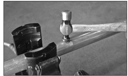
FIGURE 10a: Peen edge of filler hole over top surface of plug.
