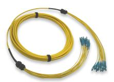
RUF1SCSC20M-12-3581 SC — SC 12 fibre singlemode pre-terminated riser cable 20 m, 500 mm breakouts with 3 mm yellow zero fibre oversleeving both ends, cable glands both ends
