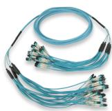
RMB4LCLC5M-48-3H11 LC-LC 48 F OM4 pre-terminated bundled round mini 5 m, 500 mm breakouts with 2 mm duplex zero fibre oversleeving both ends.
