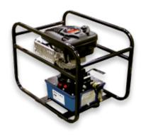
The 30GBM is a gas powered pump that produces 10,000 PSI of hydraulic pressure. It is designed to operate any 10,000 PSI compression tool. The two-stage pumping system allows for rapid ram advance. The "suc-o-matic" valve helps tools retract faster. The manual control has three settings: advance, hold and retract. The 30GBM is designed for continuous duty.
