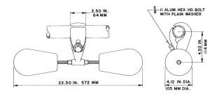
AFL Highway Truss Dampers offer the most practical and economical solution for vibration problems normally encountered in highway sign trusses. The AFL 1708-17.1 damper, weighing 31 lbs. (14.06 kg), is the size most commonly used for highway truss applications. A single damper located at the mid-point of the truss will provide vibration protection for lengths between 60 and 140 ft (18.3-42.7 m). Special consideration should be given to longer spans or cantilever applications.
