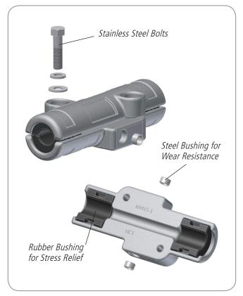
The HIBUS Series Conductor Trunnion is designed to reduce static and dynamic stress at the attachment point on transmission conductors without the use of armor rods or line guards. Rated for 250°C operation, the HIBUS Series Conductor Trunnion has a specially formulated bushing material for high temperature conductors.
