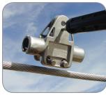
3. With the HIBUS Suspension in the open position, locate the unit on the conductor
