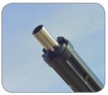
6. Attach a "Drive Socket" to the "Hot Stick" (normally included with standard hot stick kits)
