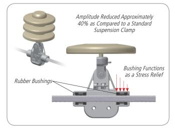
The HIBUS clamp is designed to reduce static and dynamic stress at the attachment point on transmission conductors without the use of armor rods or line guards. Rated for 250°C operation, the HIBUS clamp has a specially formulated bushing material for high temperature conductors. The hinged concept on the suspension configuration provides self-alignment of the housing halves. All hardware is captive except for the mounting pin.
