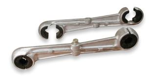
Spacers are necessary on horizontal bundle construction to prevent damage from wake-induced oscillation, ice unloading and short circuit clashing. AFL's Speed-Grip Spacer employs elastomer bushed clamps to firmly grip the conductor. It is specially designed to allow rapid installation without special tools.
