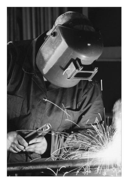
Welding of aluminum in electrical construction offers a superior and economical means of joining conductors. Electric arc welding using an inert gas shield produces mechanically and electrically sound joints requiring no flux or special surface preparation other than the cleaning of the surface to be welded.
