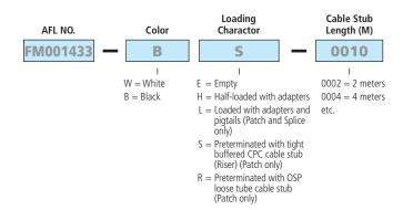
**Example:** Order number for a panel Black in color, loaded with 24 PSC adapters (4 six packs), connectors and a cable stub 10 meters in length.
