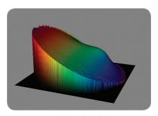
Reconstructed end-face surface of a cleaved 400 µm fiber (center cleave angle about 0.16°), with height scaled three hundred times to bring out surface irregularities and facilitate easier cleave quality analysis.
