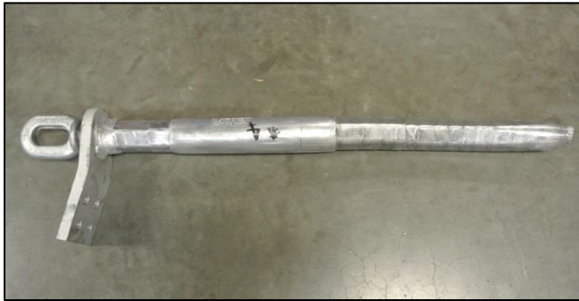
Figure 6 – Sample #4 (Test Deadend after test)
