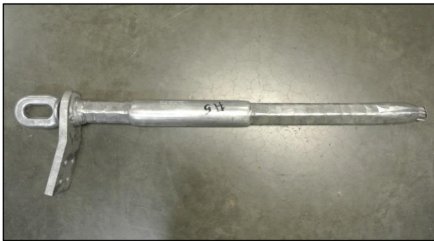
Figure 7 – Sample #5 (Test Deadend after test)
