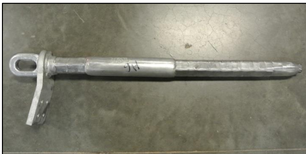
Figure 8 – Sample #6 (Test Deadend after test)
