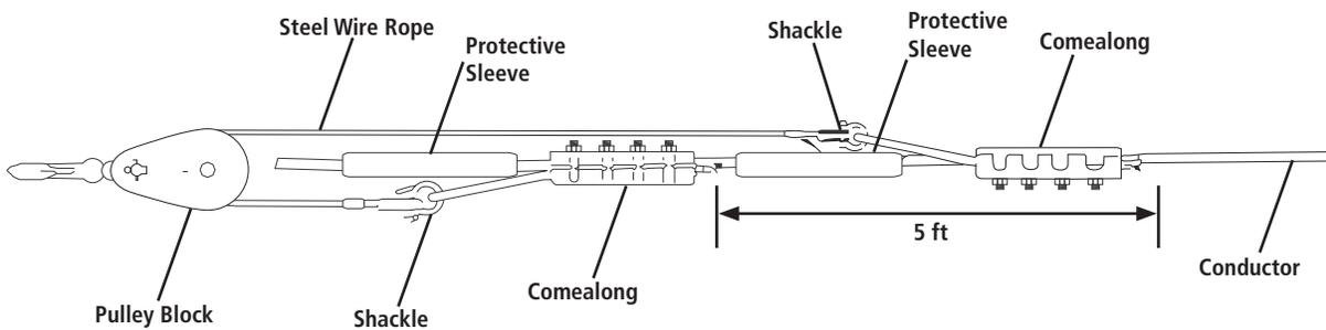
**LOAD RATING:** Maximum tension limit is 50% of the rated strength of the OPGW or 5,000 pounds, whichever value is smaller.
