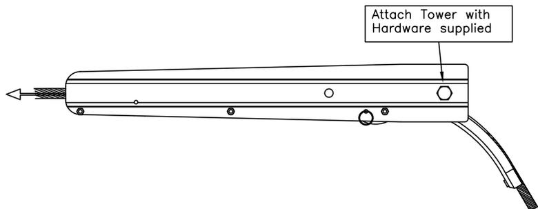
12. Form cable into the groove of the Cam/Cable Guide, then attach keeper (Item 8) with lockwashers and green break-away bolts alternately tightening bolts by 2 ft.-lbs. Repeat until break-away head breaks off. Care should be taken during installation to maintain the keeper squarely on the conductor with equal clearance on both sides of conductor.
