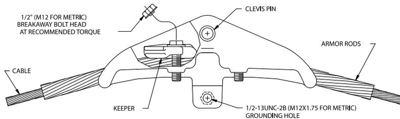
9. Attach grounding lug to grounding pad on bottom of suspension clamp (using 1/2"-13 or m12x1.75 Thread tapped hole) if grounding is required. Ground wire assembly must be long enough such that 12" of free slack wire extends directly down from the suspension grounding pad before looping back up to the adjacent structure attachment point.
