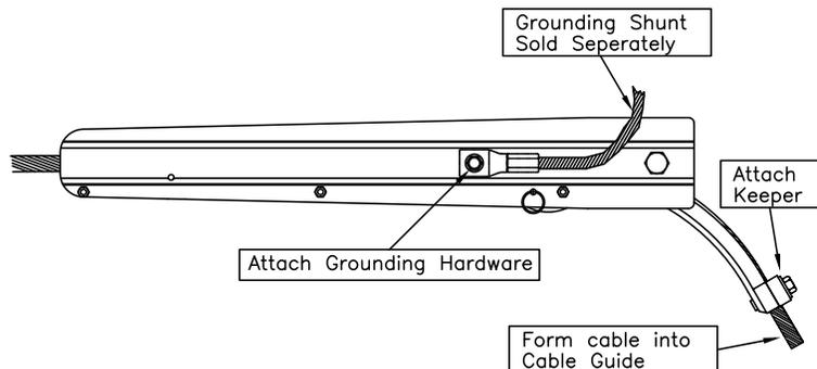
13. Attach grounding shunt with hardware provided. Torque bolts to 25 lbf.-ft. (34 N.m)
