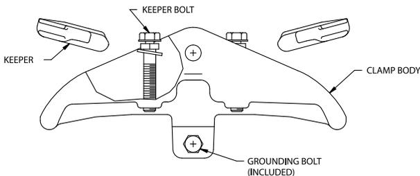
4. Place clamp body on OPGW cable and center clamp on armor rod center mark.
