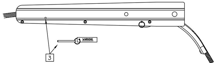
11. Attach OPGW Wedge Dead End to the tower with bolt, nut, and cotter pin supplied. Release tension on comealong. The wedges (Items 1 & 2) will advance, gripping the cable securely.
