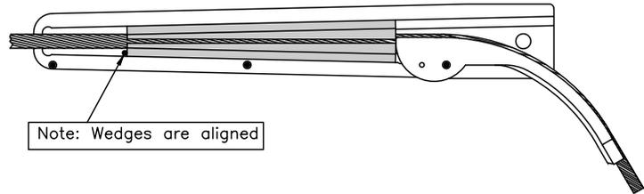
9. Replace Cable Guide Retaining Pin (Item 5) in "Location 2".
