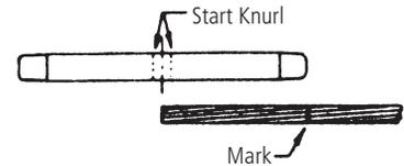
2. Mark the conductor from the end, a distance equal to half the length of the joint.
