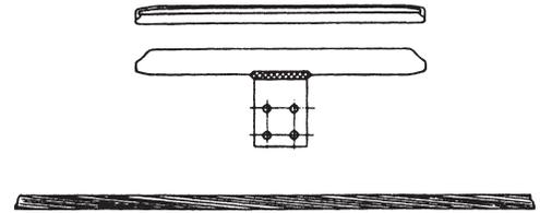
5. Place run groove on conductor and slide the keeper in place.
