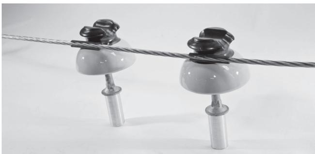
3. Install the Double Side Tie around the neck of the insulator. Ensure the leg of the tie with the crossover marking is on the same side as the conductor. Pull the tie snug against the insulator neck so that it will be properly seated.
