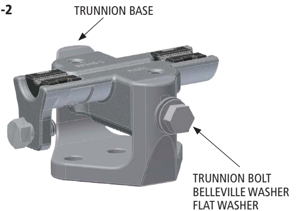
HIBUS OPGW TRUNNION BASE SHOWN INSTALLED TO TRUNNION MOUNTING BRACKET
