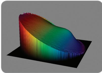
Reconstructed end-face surface of a cleaved 400  $\mu\text{m}$  fiber (center cleave angle about 0.16°), with height scaled three hundred times to bring out surface irregularities and facilitate easier cleave quality analysis.
