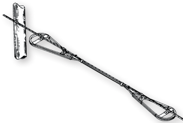
Reserve Cable Storage
