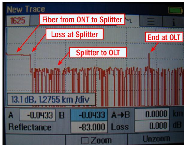
Figure 3: FTTx In-Service Mode provides OTDR trace only as far as the Splitter
