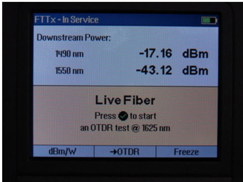
Figure 7: Live fiber detected; Press Test
