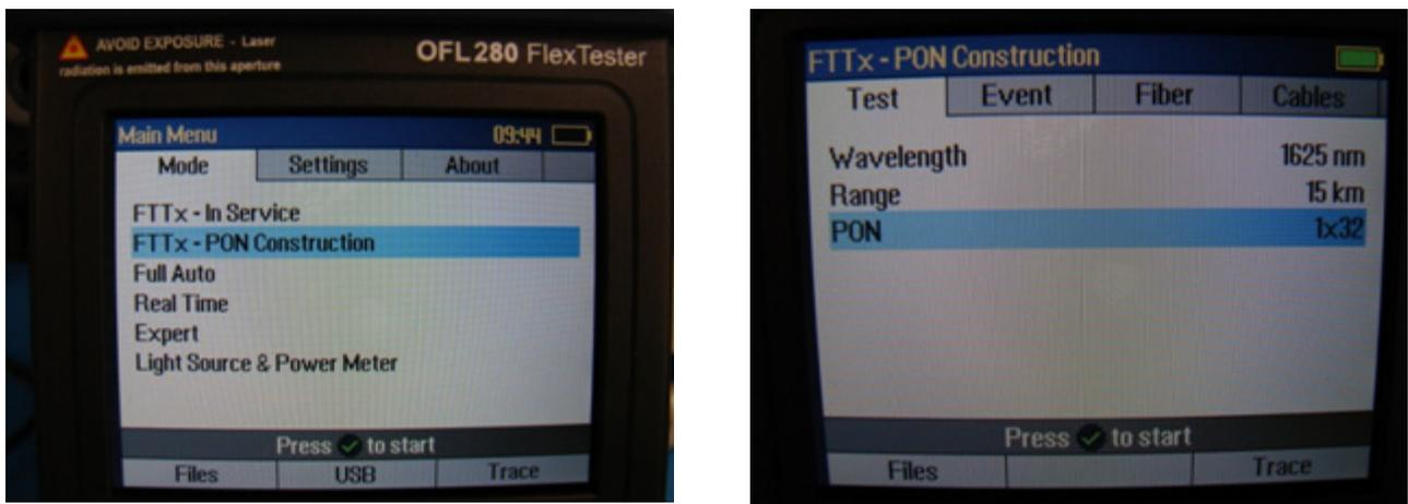
Figure 4: From Main Menu (Left) Select FTTx – PON Construction Setup (Right)
