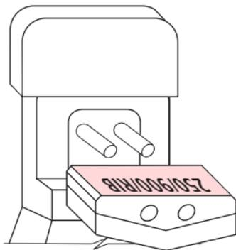
The "250/900/RIB" side faces out for the 250  $\mu\text{m}$  and 900  $\mu\text{m}$  coated and ribbon fibers testing
